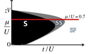
**Figure 2.** Schematic zero-temperature phase diagram. Schematic of the conventional zero temperature mean field phase diagram of Eq. (1) at density below one with no disorder. By fixing the chemical potential to be  $\mu/U=0.7$  and increasing the hopping from zero we traverse the phase diagram through the solid, supersolid, and superfluid phases, respectively<sup>11,14</sup>.
